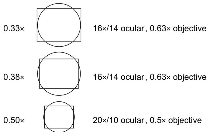
Figure 5. Compensating with smaller ocular view field. Circles and rectangles represent microscope and  $\frac{1}{3}$ " camera views with the indicated coupler magnification (left) and ocular (right). Note that low-magnification objectives increase the working distance (double for 0.5 $\times$ , 1.6 $\times$  for 0.63 $\times$ ).
