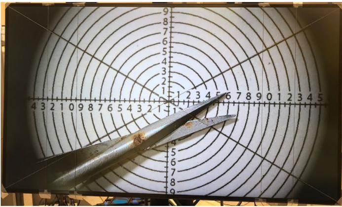
**Figure 3.** Phototube FOV. Photographed on a monitor connected to the camera via HDMI, this corresponds to the microscope ocular FOV in Figure 1A. The circular FOV is larger (28.5 mm diameter) than the ocular view field of 23 mm but is dim at the edges. Barely visible are threads taped to the monitor, showing square and 4:3 cropping.
