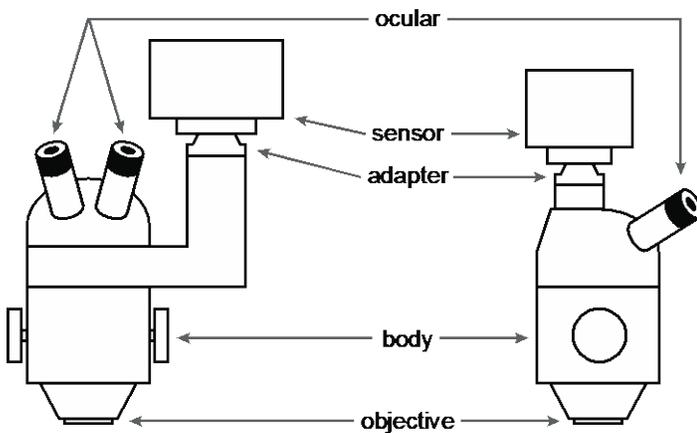
**Figure 2.** Variables affecting FOV. Ocular view diameter affects microscope FOV. Sensor size and coupler magnification affect camera FOV. Microscope body and objective magnification affect both views equally.
