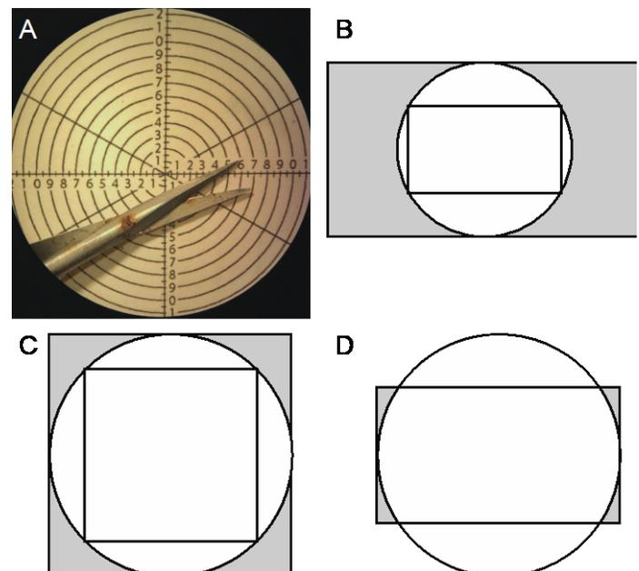
**Figure 1.** FOV tradeoffs. **A.** Photograph taken through the ocular, showing the circular FOV. **B.** Capturing the entire FOV (outer rectangle) vs. avoiding any blank space (inner rectangle); a 16:9 sensor aspect ratio is assumed. **C.** Cropping to a square can capture the entire field (outer square) or completely avoid blank space (inner square); an intermediate may be best. **D.** One possible compromise view for live streaming.
