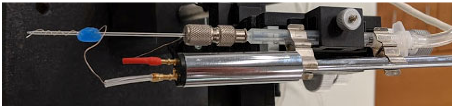
Figure A1. Assembled suction electrode. Refer also to Figure 1 in the text.
