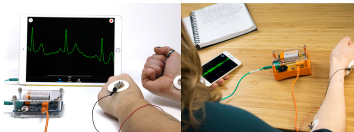
Figure 2. Left: Heart & Brain SpikerBox for recording EEG, EOG and EKG signals. Right: MusclePro SpikerBox for capturing EMG signals.
