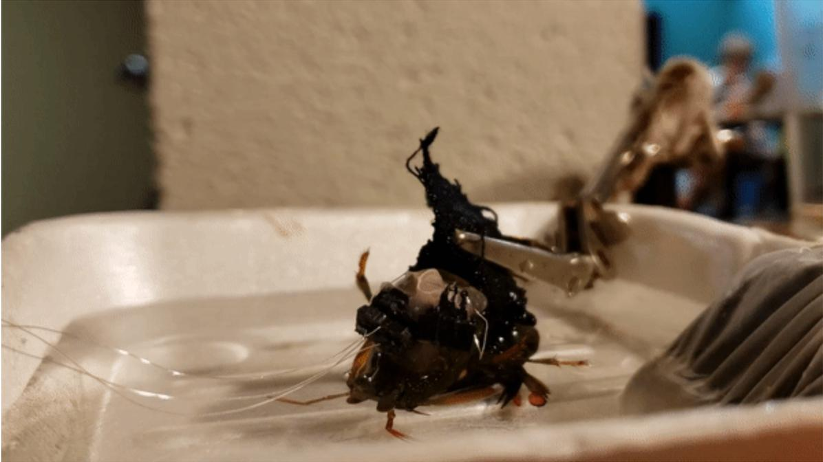
7. Make sure both channels are working, the Backyard Brains app running, and that you have a way of presenting stimuli. Grasp the backpack on the animal's carapace and plug in the cable, making sure the ground lead of the cable goes into the ground socket, which should be on the side. It may take a few tries to grasp the backpack firmly and plug the probe in.
