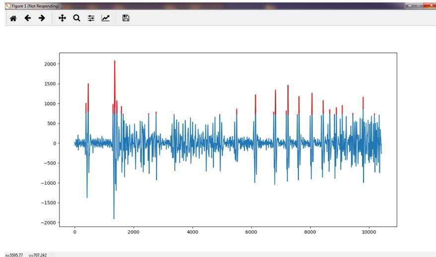
Another window will pop up with a visualization of your EMG region, as above. Now, you have to isolate each spike to collect its waveform, without including noise. To do that, this script uses a technique called thresholding to find “threshold crossings” that only include the tips of spikes. From there, the program isolates the points around the spike and stores it for later analysis.
