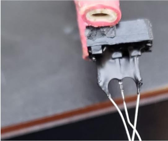
4. To make the plug and microphone, cut off the alligator clips and strip the ends of the wires on each of the Backyard Brains [muscle electric cables](#).
