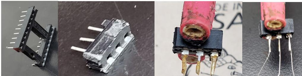
3. Use liquid electrical tape or your preferred method of insulation, cover the exposed leads, it will take at least 10 minutes to dry. Make sure the entire insulated length is covered. If metal is
