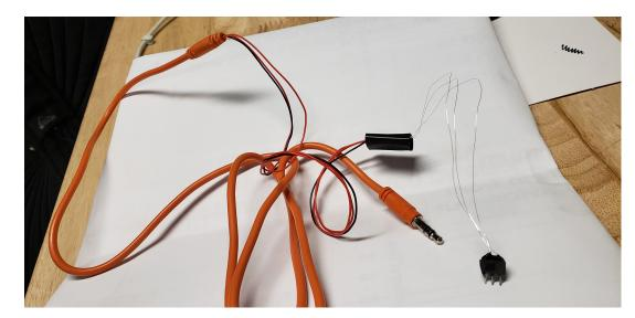
8. Insulate all exposed metal and solder with liquid electrical tape.
