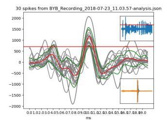
The main figure is a summary of all the spikes, with each in grey, the average in red, and one standard deviation plotted in green. In the top right, we see all the spikes together in the trace, and on the bottom right, we see what thresholding the audio and artifact has created: two cross shapes, which tell
