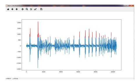
Another window will pop up with a visualization of your EMG region, as above. Now, you have to isolate each spike to collect its waveform, without including noise. To do that, this script uses a technique called thresholding to find "threshold crossings" that only include the tips of spikes. From there, the program isolates the points around the spike and stores it for later analysis.
