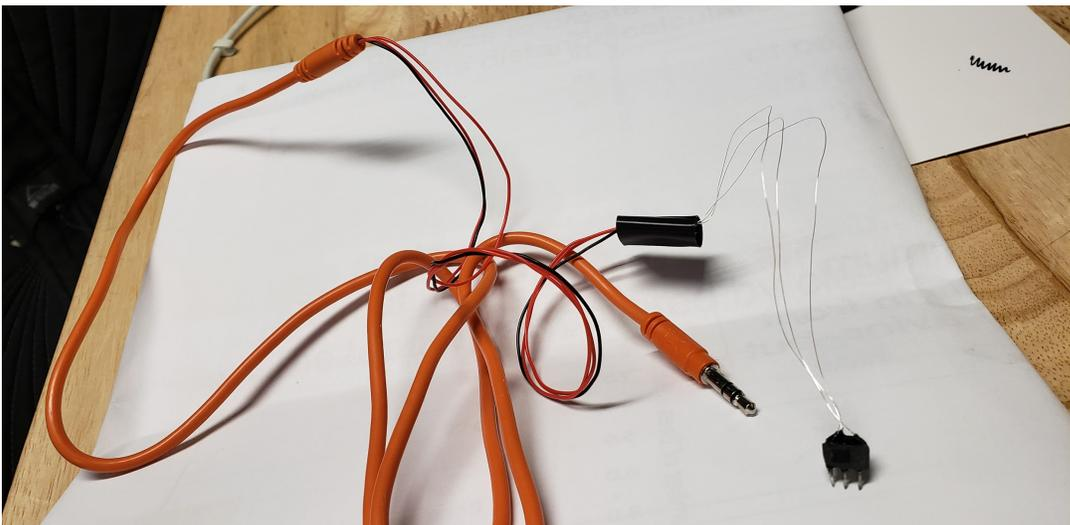
9. To make the microphone/hydrophone, strip the microphone so that it looks like it does below. Solder one red wire to each, and solder the black wire to one of them. This allows the hardware on the Spikerbox Pro to function as a simple microphone.
