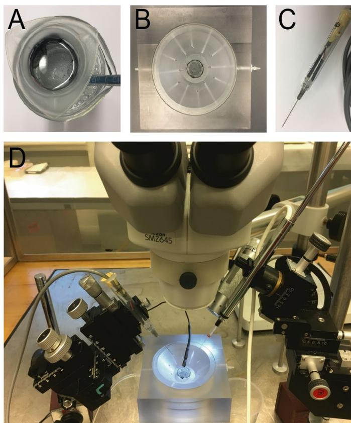
**Figure 1.** In-house made equipment and rig setup. **A.** Slice keeper with nylon bottom immersed in bubbling ACSF. **B.** Recording chamber with elevated, nylon-covered stage. ACSF flows into bottom of chamber (from left) and out from top of chamber (from right). **C.** Bipolar stimulating electrode. **D.** View of the rig with stimulating electrode (left) and recording electrode (right) mounted in micromanipulators and placed above recording chamber containing a bath ground (center).
