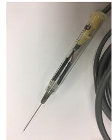
Recording electrodes (bubble test: right)
