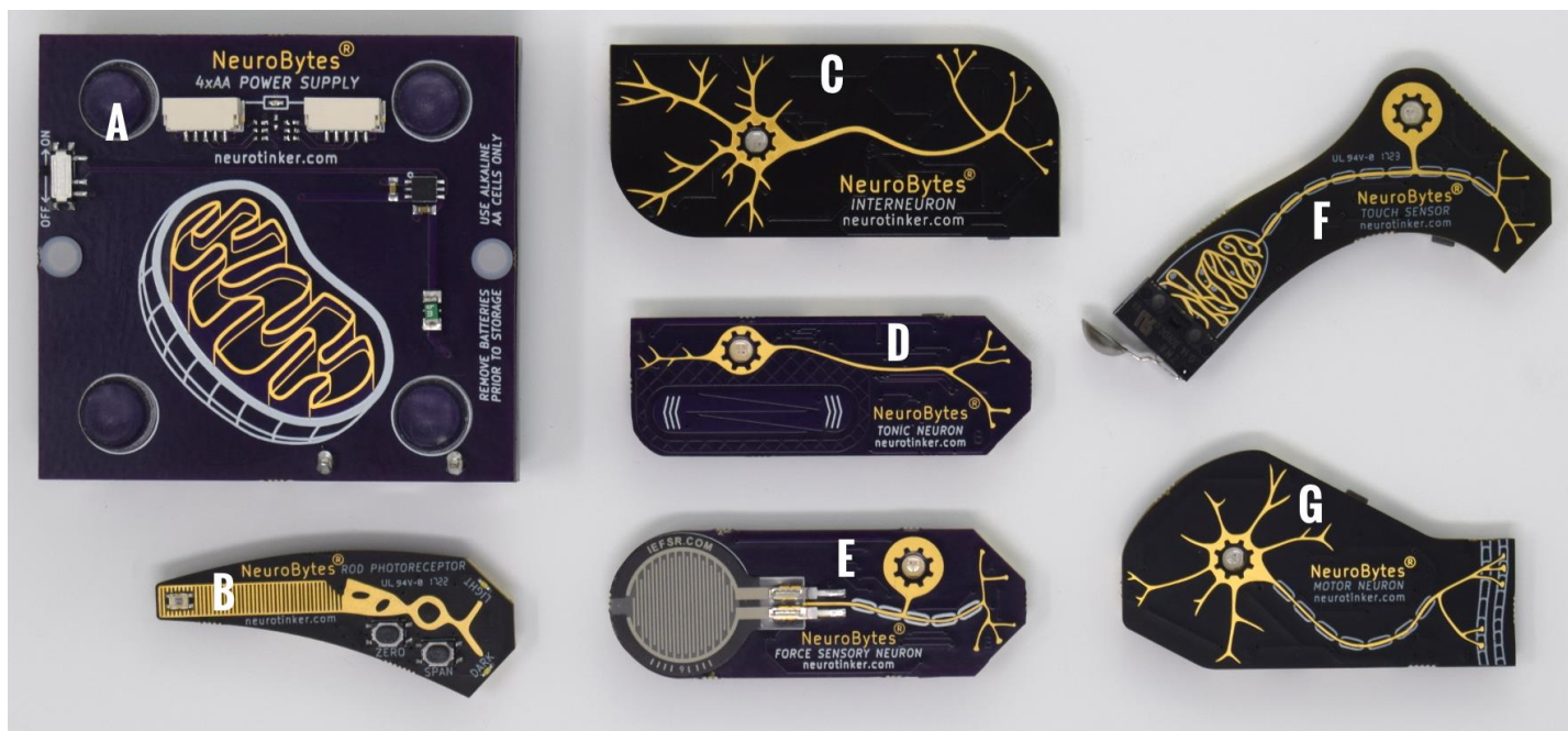
Figure 4. The NeuroBytes Neuron Simulator Ecosystem. (A) Battery pack. (B) Rod Photoreceptor. (C) Interneuron. (D) Tonically Active Neuron. (E) Pressure Sensory Neuron. (F) Touch Sensory Neuron. (G) Motor Neuron.
