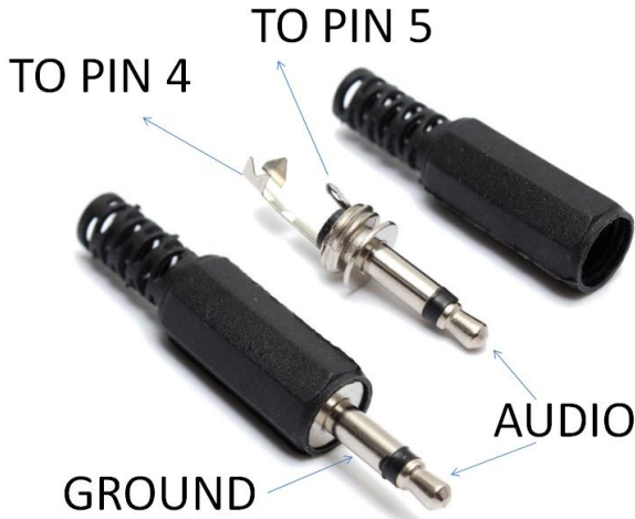
Figure 3. Pin layout of a mono audio connector that plugs into the USB sound card. The tip is connected to the negative end of the electrolytic capacitor whose positive end is connected to in 5 of the LM386 chip. The sheath is connected to the blue rail.
