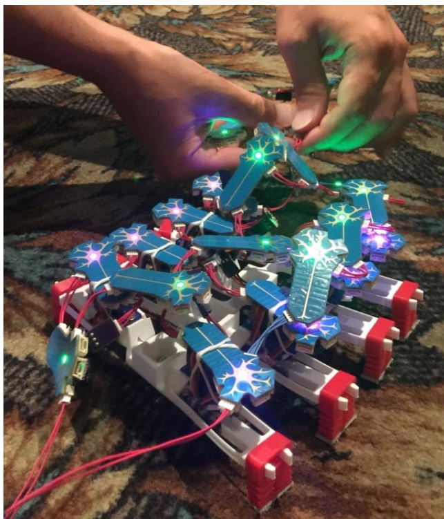
Figure 5. Central Pattern Generator based NeuroBytes circuit driving walking behavior in a model insect.
