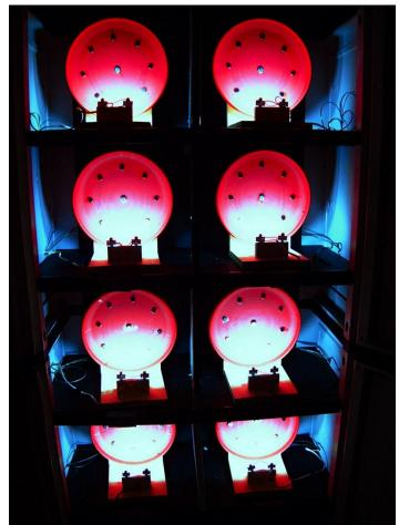
*Figure 2.* Earthworm Running Wheels in Enclosure, Eight running wheels housed in plastic utility cabinet. When doors are closed each wheel is in the dark, and is isolated visually from the other wheels.
