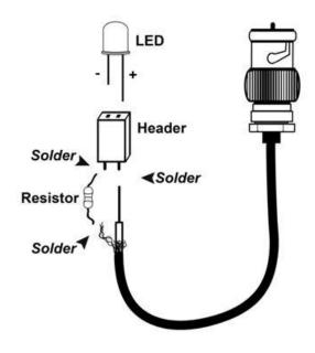
*Figure 2.* Schematic of the LED light stimulus assembly. A standard BNC and components are soldered together as indicated by arrows.
