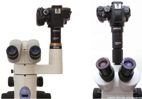
Figure 1. Microscopes and adapters. Left: phototube with adapter and dSLR. Right: trinocular microscope with adapter and dSLR. Images courtesy of Micro-Tech-Lab, www.LMScope.com .
