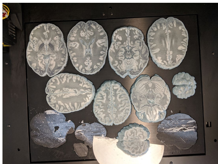
Figure 1. Polyjet printed axial slices being removed from the build plate.
