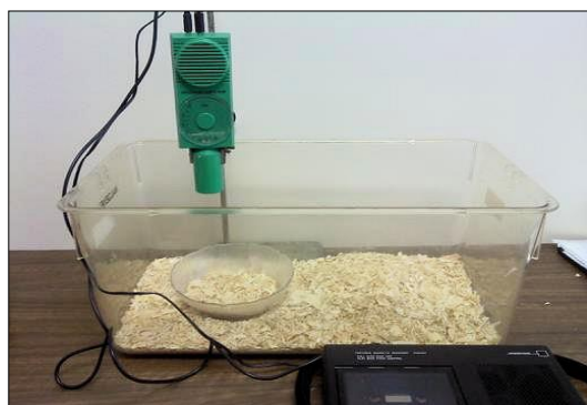
Figure 2. USV testing chamber. The ultrasonic bat detector is set up directly above a small enclosed area in which the pup should be placed, to ensure the pup stays directly under the detector. A heating pad should be placed under the cage to ensure that the pups will not become hypothermic while separated from the dam and litter.
