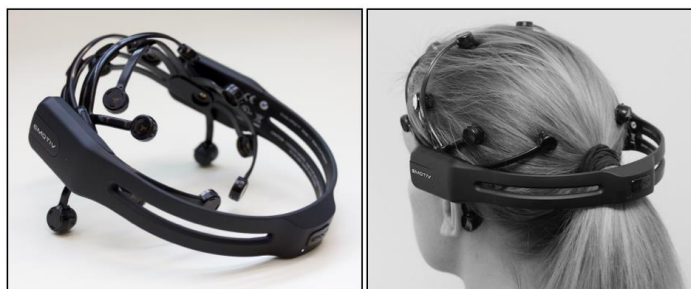
Figure 1. EMOTIV EPOC+ EEG system. Left panel: EMOTIV headset. Right panel: EMOTIV headset as worn by participant.
