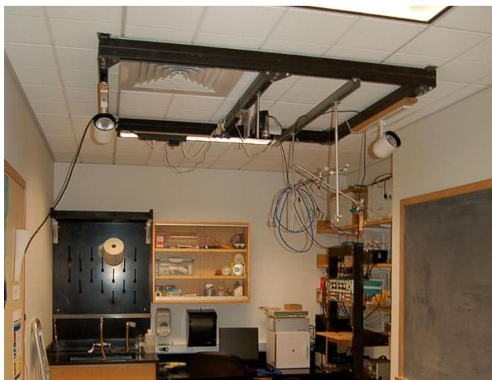
*Figure 7.* Metal framing support system suspended from the ceiling in a recording area of an electrophysiology laboratory. In this example, lights, a commutator, and a video camera are securely attached to the system. (Hamilton College).
