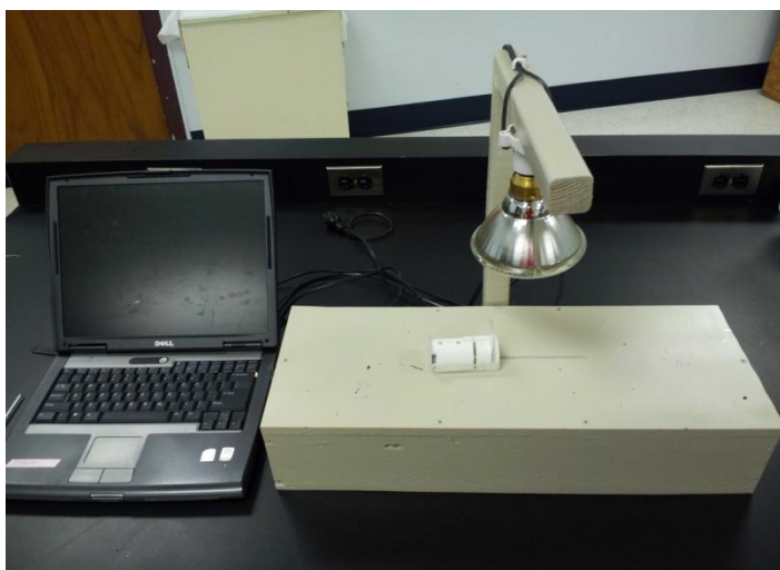
Figure 1. Photograph of the tail flick apparatus and controlling computer. The circuitry is attached under the mouse platform.
