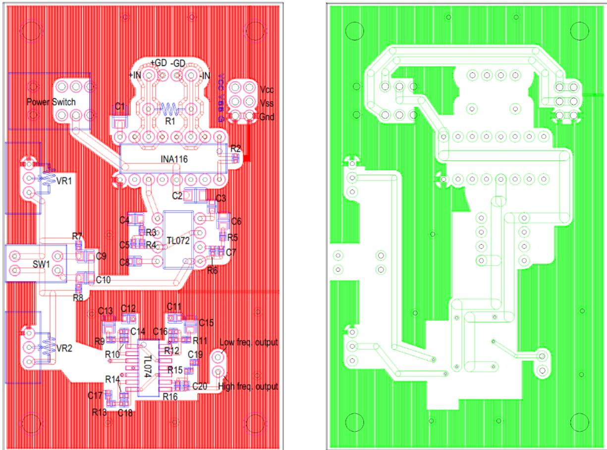
Figure 2. The printed circuit board (PCB). *Left*: the front surface and the electronic parts. Through holes labeled as +IN and -IN are, respectively, connected to positive and negative inputs, and +GD and -GD are connected to their shield conductors. Vcc and Vss are positive and negative DC power supplies. *Right*: back surface. The part numbers correspond to those in Figure 1.
