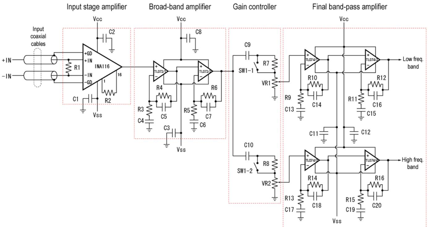
Figure 1. Circuit diagram. See Table 1 for the list of the electronic parts.
