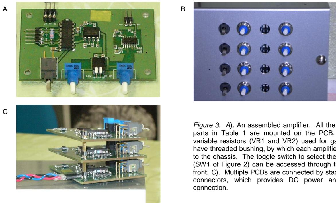
Figure 3. A). An assembled amplifier. All the electronic parts in Table 1 are mounted on the PCB. B). The variable resistors (VR1 and VR2) used for gain control have threaded bushing, by which each amplifier is bolted to the chassis. The toggle switch to select the max gain (SW1 of Figure 2) can be accessed through the hole in front. C). Multiple PCBs are connected by stack-through connectors, which provides DC power and ground connection.
