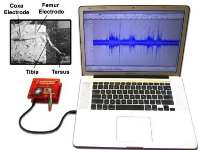
Figure 2. Standard setup of the bio-amplifier plugged into the line input of the laptop computer. Inset: example of electrode position for cricket leg action potential recording from the femur.
