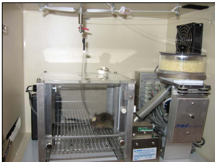
Figure 18. Mouse with head stage connected to microdialysis apparatus. Lengths of connector assembly pertain to distances between fluid swivel and animal.
