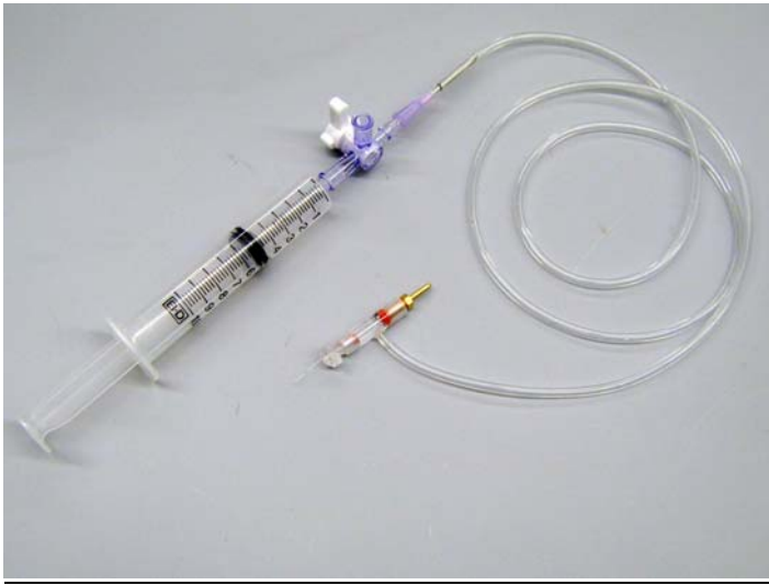
Figure 3. Assembled suction components of the electrode. See Fig. 1 legend for parts identification.
