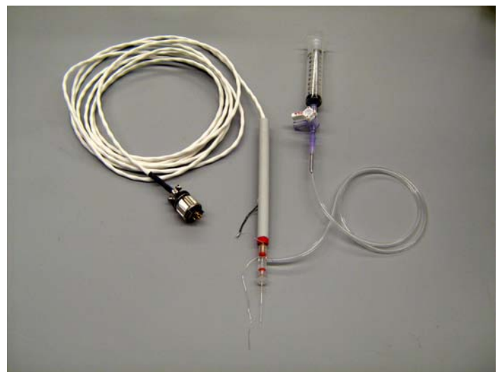
Figure 4. Completed suction electrode. See Fig. 1 legend for parts identification.
