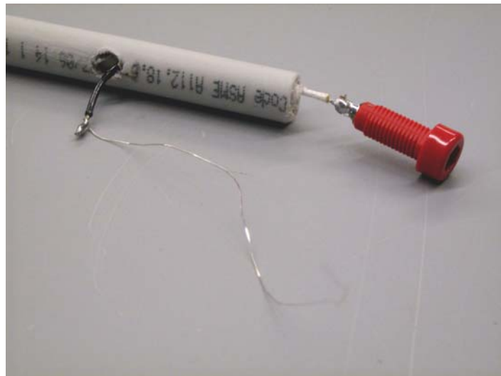
Figure 2. Electrode handle showing 5 mm hole for external reference wire soldered to silver wire lead, and pin jack soldered to the internal (white) amplifier.
